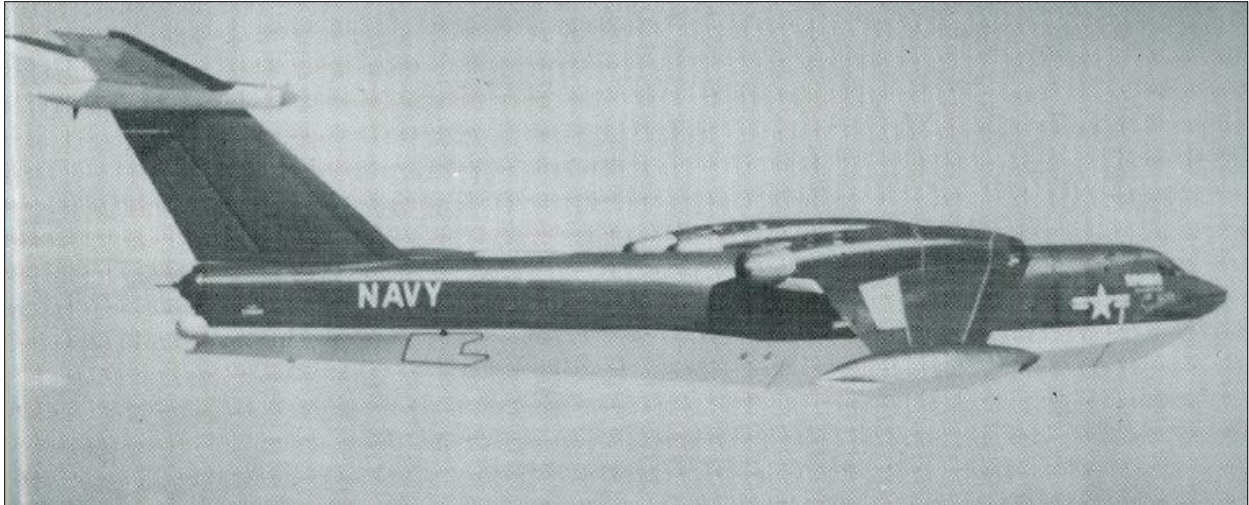
Figure 8: Image of P6M (SeaMaster) jet seaplane in flight. (Source: Town of Hertford Bi-Centennial, p. 63, 1958).
